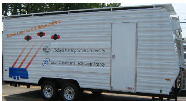
Fig.2 The 1.6 \mu\text{m} CO 2 DIAL container.
