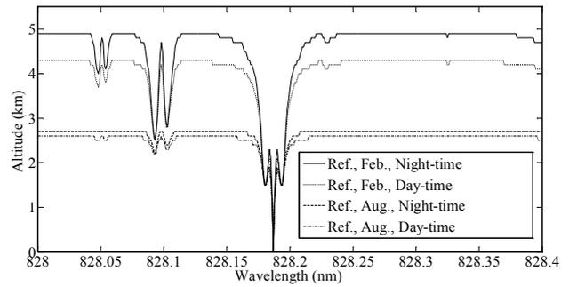
Fig. 7. Maximum reached altitude according to the RMSE of less than 10% for the pair of referenced online-wavelength (828.187 nm for both February and August) and varied offline-wavelength (from 828 nm to 828.4 nm) during day-time and night-time, respectively.
