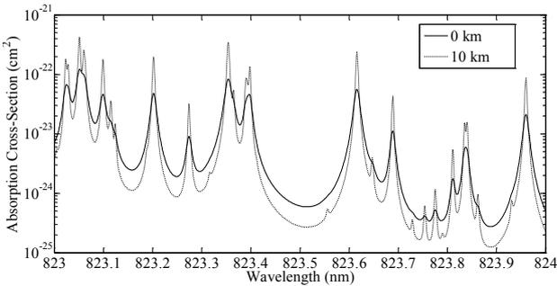
Fig. 3. Voigt profile of the water vapor absorption cross section around the selected operational lines at the altitudes of 0 km (solid line) and 10 km (dotted line), respectively.
