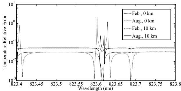
Fig. 4. Temperature relative error of the pair of the online-wavelength (823.616 nm for February and 823.689 nm for August) and varied offline-wavelength (from 823.4 nm to 823.8 nm) at the altitudes of 0 km and 10 km, respectively.
