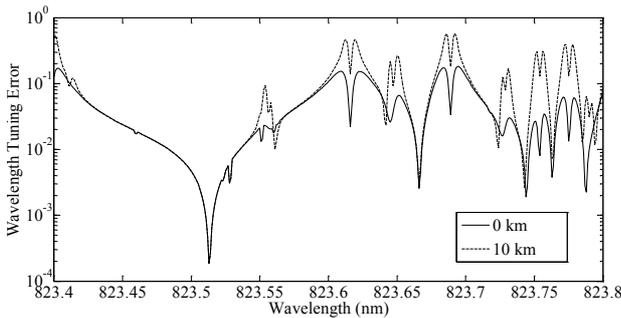
Fig. 5. Wavelength tuning error around the selected operational lines at the altitudes of 0 km (solid line) and 10 km (dotted line), respectively.
