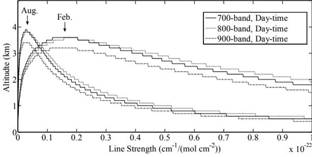
Fig. 2. Maximum reached altitude according to relative error of less than 10% for 700nm-band (solid line), 800nm-band (dotted line), and 900nm-band (dash-dot line) during day-time of February and August, respectively.
