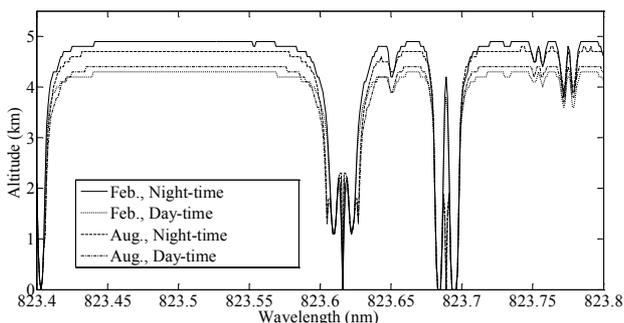
Fig. 6. Maximum reached altitude according to the RMSE of less than 10% for the pair of online-wavelength (823.616 nm for February and 823.689 nm for August) and varied offline-wavelength (from 823.4 nm to 823.8 nm) during day-time and night-time, respectively.
