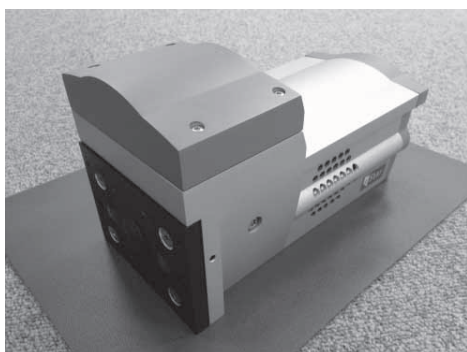
Figure1 Photograph of an intensified CCD camera with gating system, DH734I-18F-03 made by ANDOR, for the monitoring system.
