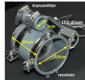
Fig. 1. LED mini lidar in biaxial configuration with angle adjuster configured for near-range ground observation.
