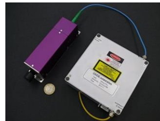
Fig. 3. Frequency converter laser of 355 nm by utilizing PP-LBGO device
