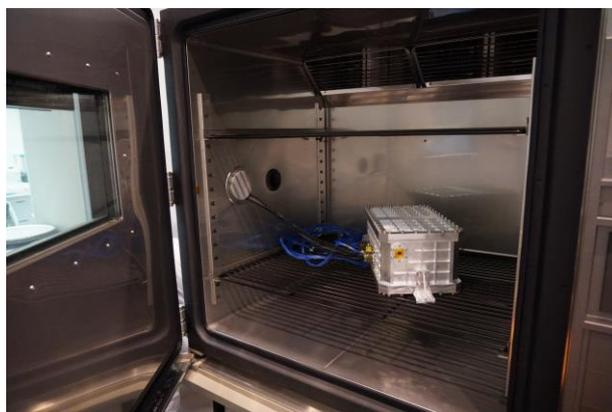
Figure 3. pressurized laser canister in constant temperature bath.
