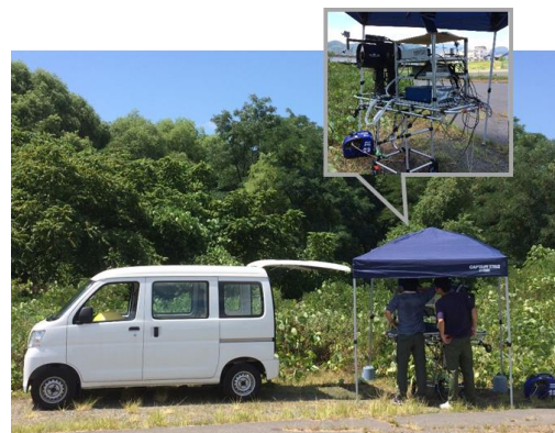
Fig.1 Observation of plant fluorescence in vegetation using a LIFS Lidar
