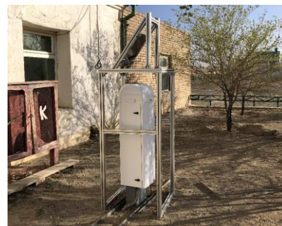
Figure 2: Picture of the ceilometer (Vaisala CL51) and mirror mount in Dalanzadgad, Mongolia.
