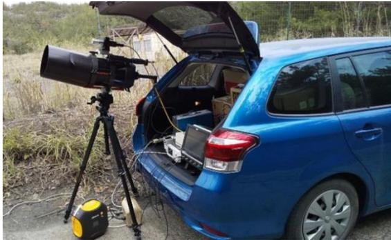
Fig.2 Developed portable particle counting lidar.
