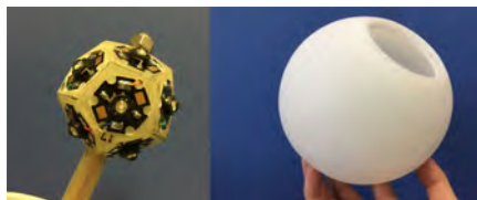
Fig.3 UV LEDs on a dodecahedron to achieve isotropy of light. Covering LED with the Diffuser creates a pseudo light ball.
