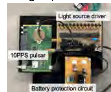
Fig.4 Light source circuit to control light intensity, pulse width, and frequency.
