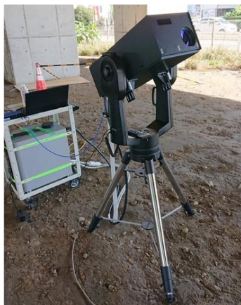
Fig. 1 (Left) Portable remote LIBS system and (Right) optical layout of the LIBS system.
