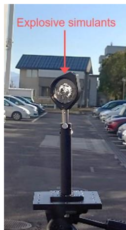
Fig.2 Installation situation of explosive simulants.
