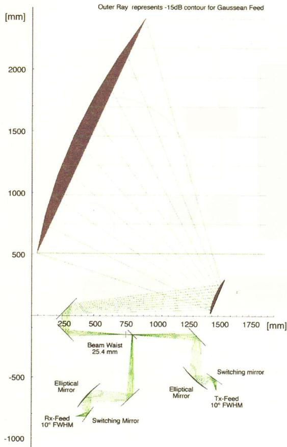
**Fig. 3: Schematic layout of the quasi-optical frontend and antenna**
