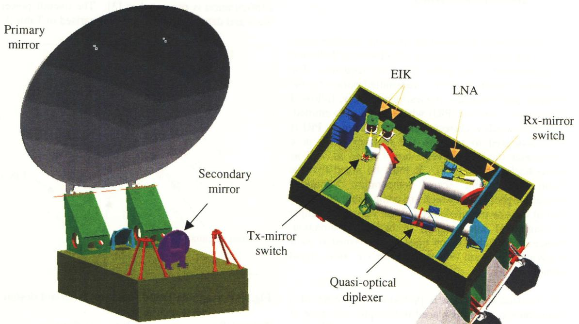
Fig. 2: CPR instrument configuration (left) and inside view (right) with quasi-optical beam path (-40 dB contour in white)
