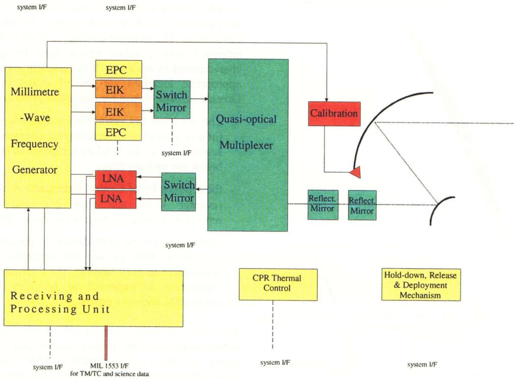
Fig. 1: CPR functional block diagram
