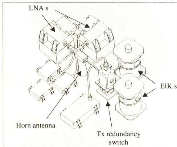
**Fig. 4: Waveguide-based (backup) frontend design**
