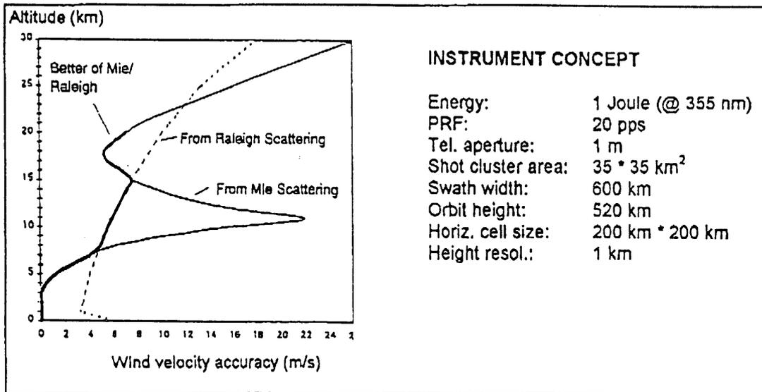
Fig.3: Velocity accuracy measurements vs. altitude employing either Mie and/or Rayleigh returns at 355 nm
