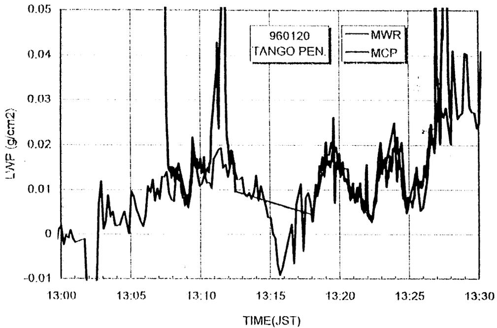
Comparison of cloud liquid water path (LWP) from nadir radiance measurements with a dual-frequency microwave radiometer (MWR) and flux reflectance measurements with MCP, on board C404 flying at the altitude of 3000m, on 20 January 1996.
