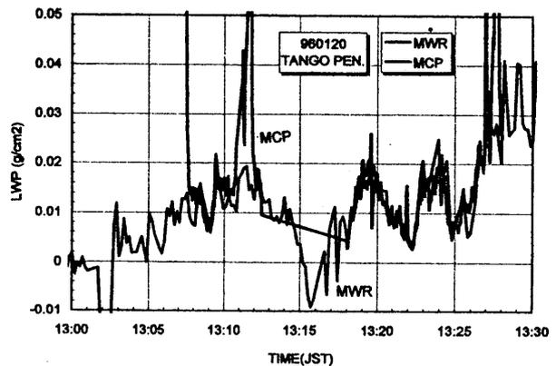
Fig. 5. Comparison of cloud liquid-water-path (LWP) measured by a dual-frequency microwave radiometer (MWR) and estimated from the spectral solar reflectance measured by the multichannel cloud pyranometer system (MCP), on board C404 flying at the altitude 3000m, on January 1996.
