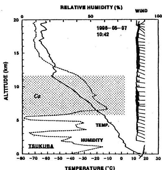
Fig. 1. Altitude distribution of the air-temperature, relative humidity and wind measured by a rawinsonde built in the radiation-sonde launched at 10:43(JST) on 7 May 1996.
