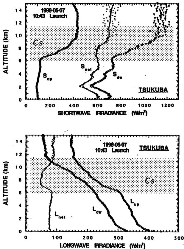
Fig. 4. Altitude distribution of the downward and upward fluxes of the shortwave radiation (TOP) and the longwave radiation (BOTTOM), respectively, measured by the accompanied radiation-sonde for the same case as Fig. 3. The net fluxes defined as differences of the upward fluxes and downward fluxes are also plotted. The solar zenith angle was about  $20^\circ$ .
