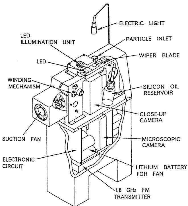
Cutout view of the new version of HYVIS (Ice-Particle-Video-Sonde) [Orikasa et al., 1996]
