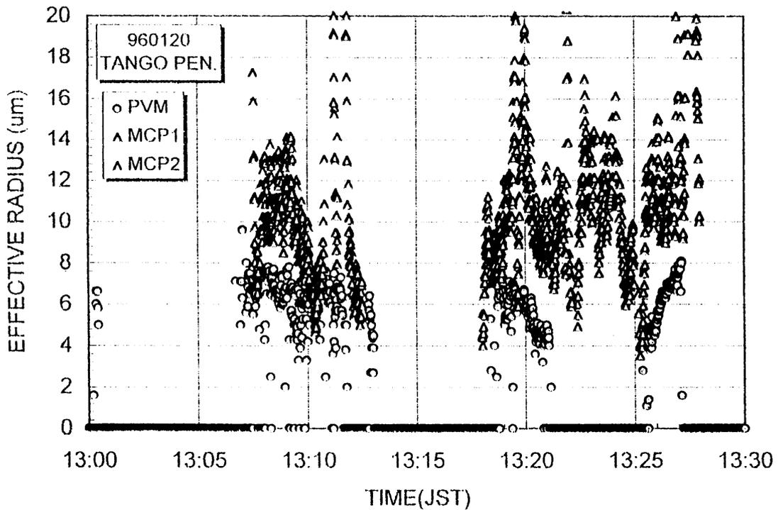
Effective radii of cloud droplets from remote-sensing with MCP on board C404 (Triangles) and in-situ measurement with PVM on board B200 (circles).
