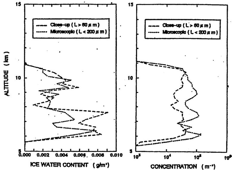
Fig. 3. Vertical profiles of the ice-water-content (LEFT) and ice-crystal concentration (RIGHT) measured by a cloud-particle-video-sonde launched at 10:43(JST) to cirrostratus cloud observed on 7 May 1996.
