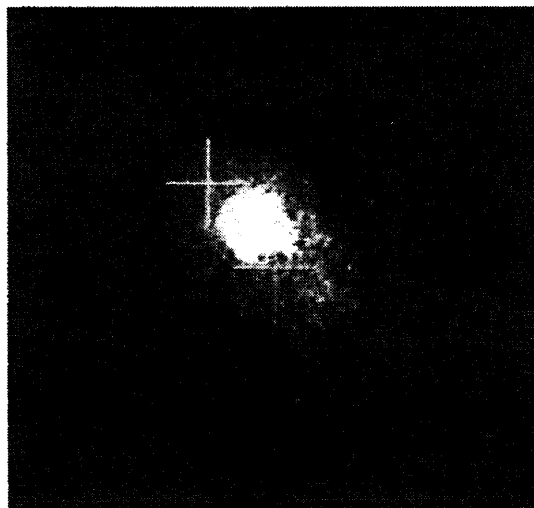
Reflection from the RIS at 532-nm taken with the ICCD camera located in Coude optics. The field of view of the ICCD is approximately 200 microradians.
