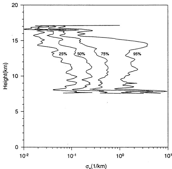
Fig. 3 One application of combined lidar and spectral thermal infrared sensing is to derive the IR absorption cross section as a function of height for cirrus. Such retrievals are not possible with passive sensing alone. The figure shows the frequency of observation as a function of altitude for tropical cirrus from ER-2 data. Each line represents the values for which the indicated percentage of cross sections were below the value.
