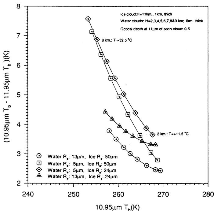
Fig. 4 The sensitivity of the split window equivalent brightness temperature of a two layer cloud system of cirrus over stratus. The split window brightness, from which particle size is often retrieved, is highly sensitive to the vertical structure of the cloud layers. The multiple layer conditions can not be retrieved from passive data.
