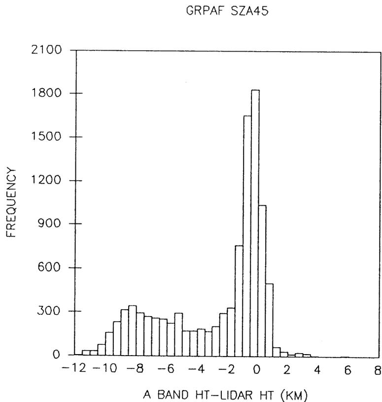
Fig. 6 A comparison of cloud heights derived from an experiment Oxygen A-band technique to direct measurements from lidar. Active measurements provide a direct means to obtain cloud height for comparison to passive retrievals.
