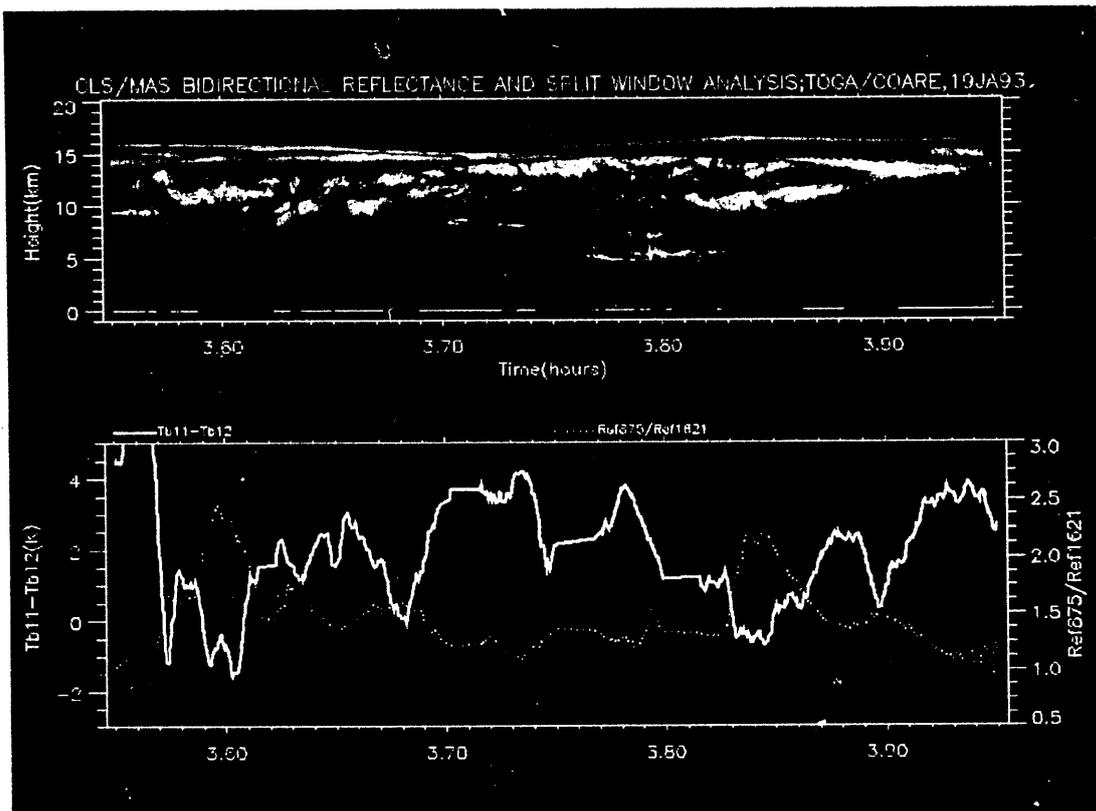
Fig. 2 Data from the NASA ER-2 high altitude aircraft showing results for combined remote sensing of tropical cirrus clouds with lidar and spectral thermal infrared measurements.
