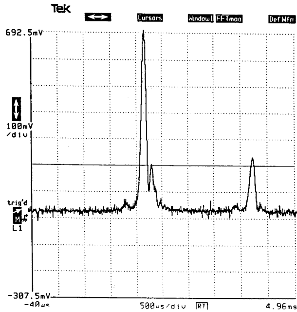
Figure 3. Laser wavemeter spectrum showing single mode, with weak second mode.
