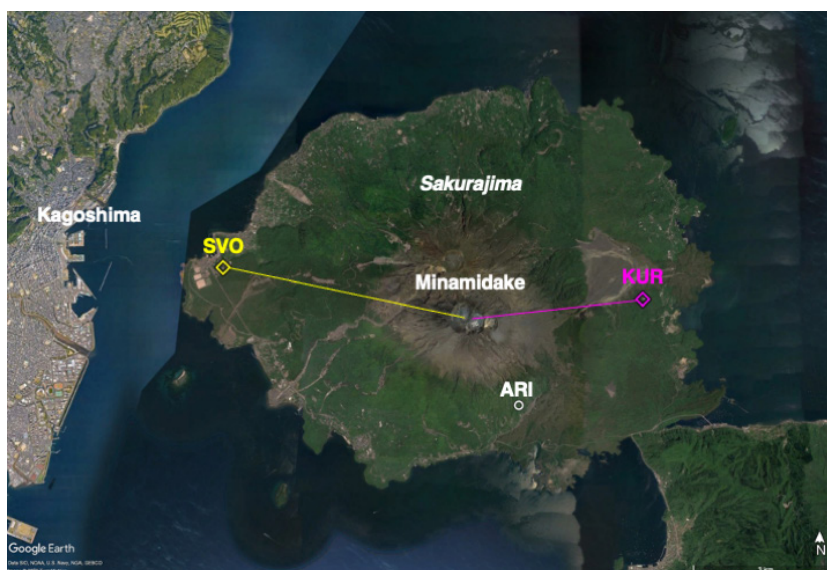
Fig. 2 Locations of lidar instruments installed at SVO (yellow diamond) and KUR (purple diamond) at the Sakurajima volcano. Lines indicate their lines of sight. The open white circle indicates an underground observation tunnel by the Ministry of Land, Infrastructure, Transport, and Tourism (ARI), in which an extension meter and a seismometer are installed.
