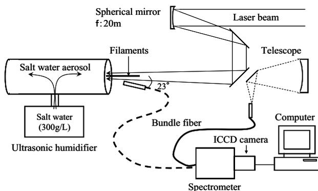
Fig. 1. Experimental setup for LIBS-LIDAR measurement of Na fluorescence from salt water aerosols irradiated with filaments generated by femtosecond laser pulses.
