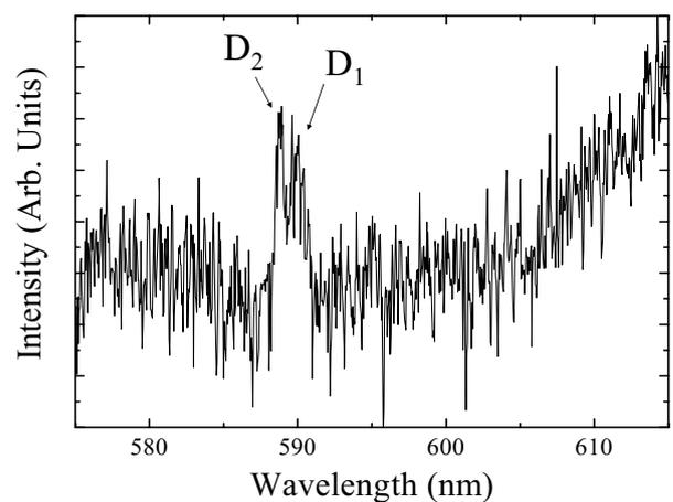
Fig. 4. Na fluorescence from salt water aerosols irradiated with filaments generated by femtosecond laser pulses measured by LIBS-LIDAR.
