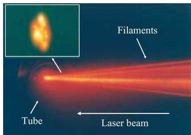
Fig. 2. Laser beam propagating around the entrance of the tube. The insert is a laser beam profile showing multiple filaments at the entrance of the tube.
