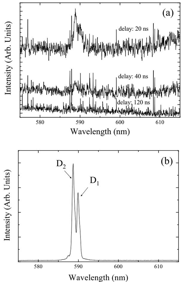
Fig. 3. Spectroscopic measurement results of Na fluorescence from (a) salt water aerosols irradiated with filaments generated by femtosecond laser pulses with delay time of 20, 40, and 120 ns from laser irradiation, and (b) spirit lamp containing salt.
