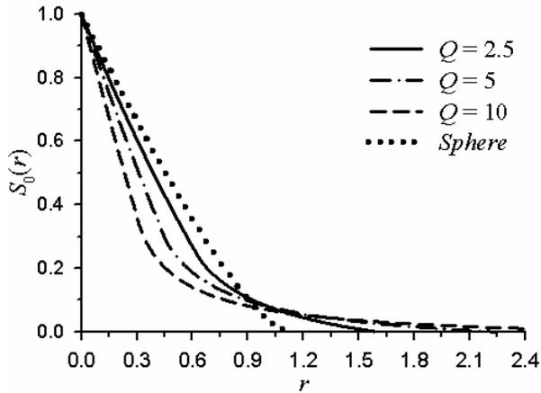
Fig.1. The shadow functions for horizontally Parry oriented hexagonal ice columns with various aspect ratios  $Q$ , where  $r = |\mathbf{R}|$ .
