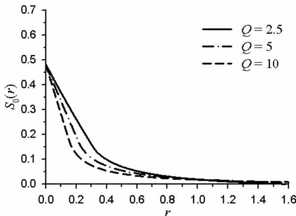
Fig.3. The shadow functions of the transmitted beams for horizontally Parry oriented hexagonal columns.
