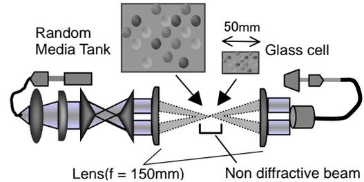
(b) Focused annular beam (Non-diffractive beam)
