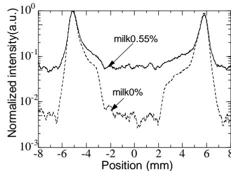
(b)Focused annular beam through the large media tank
