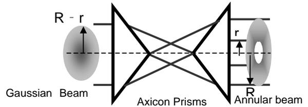
Fig.1. Transformation from the Gaussian beam to the annular beam.
