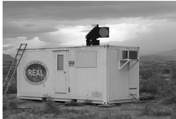
Figure 1. The Raman-shifted Eye-safe Aerosol Lidar (REAL "v1") resides in a 20-foot shipping container.
