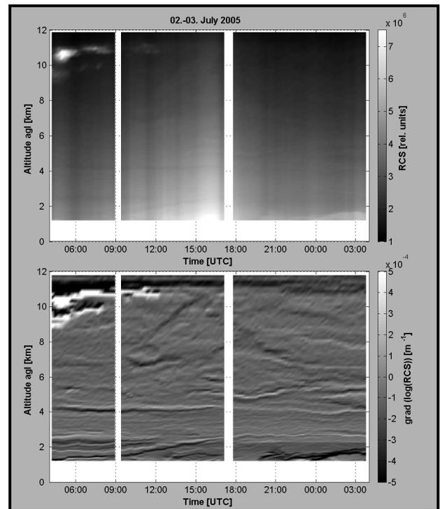
Fig. 3. Diurnal cycle of lidar observation on 2-3 July 2005. The temporal resolution is 15 minutes. The top panel shows the time-series of range-corrected signals (RCS) for the 532 nm (p) channel. The bottom panel shows the corresponding altitude log-derivative, revealing the development of the aerosol stratification. In both panels, saturated colours are used.
