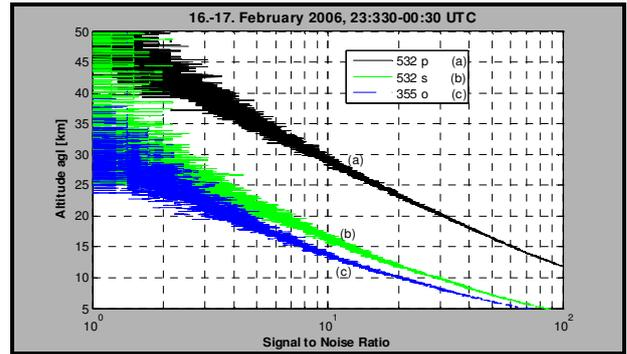
Fig.1 Signal-to noise ratio evaluated from the photon-counting data for three elastic channels. The integration time is 1 h (16.-17. February 2006, 23:30-00:30). The range resolution is 7.5 m.
