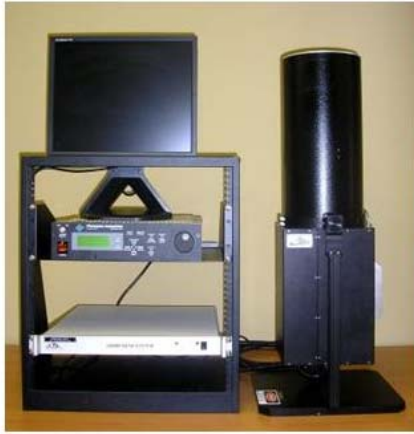
Fig. 1. (a) Left: Photograph of a MPL system (courtesy of Sigma Space). (b) Right: Optical layout of an MPL transceiver components. Dashed box shows where a Raman N 2 channel could be added by incorporation of a dichroic mirror in the existing receiver path.
