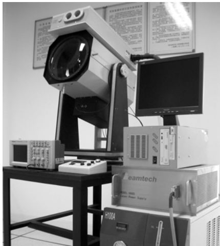
Figure 2. Mobile Scanning Lidar System Developed at Wuhan University
