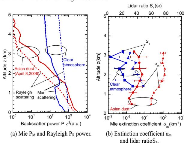
Fig. 4 Height distribution of the return signal and atmospheric optical parameters observed with averaged over 15 min. (a) is the range corrected Mie and Rayleigh backscatter power with 50 m range resolution and (b) is the extinction coefficient and lidar ratio with 300 m range resolution.
