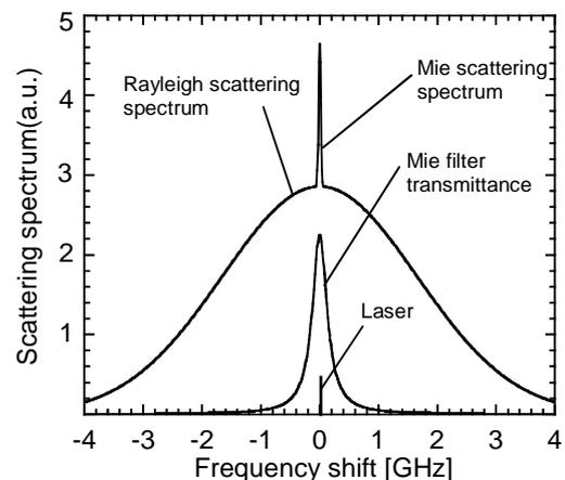
Fig. 2 Spectral profiles of the Mie and Rayleigh scattering and the filter transmittance function.
