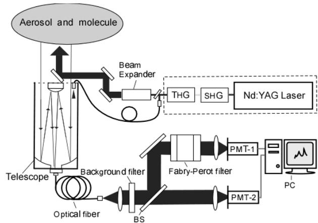
Fig. 1 Schematic of the UV-HSRL system.
