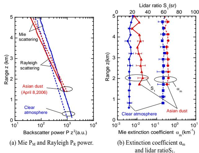
Fig. 3 Horizontal range distribution of the return signal and atmospheric optical parameters observed with averaged over 15 min. (a) is the range corrected Mie and Rayleigh backscatter power with 50 m range resolution and (b) is the extinction coefficient and lidar ratio with 300 m range resolution.
