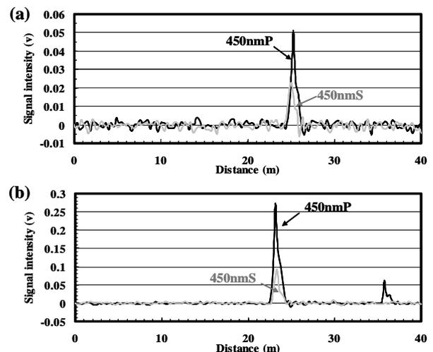
Fig. 5. Single-shot polarization signals from the paper (a) and the water droplet (b) at 450 nm depolarization channel
