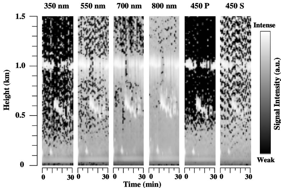
Fig. 4. Simultaneous measurements of the range squared corrected backscattered signal from atmosphere (2005/03/23 1:53~2:22 AM)
