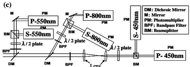
Fig. 2. Schematic diagrams of experimental setup; (a) lidar, (b) ground experiment, (c) the 3-wavelength depolarization backscattering spectrometer
