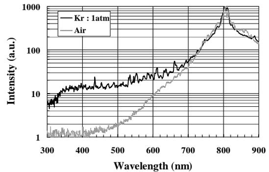
Fig. 1. White light spectra generated in atmospheric-pressure Kr and air. The laser wavelength and laser power are 800 nm and 1.0 TW, respectively.
