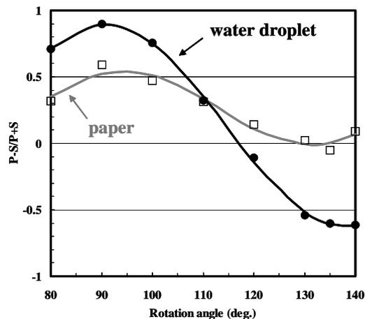
Fig. 6. Rotation angle dependence of the backscattered light from the water droplets and paper
