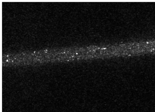
**Fig. 2 A picture image of the fluorescence emitted from the asbestos particles suspended in the vessel.**
