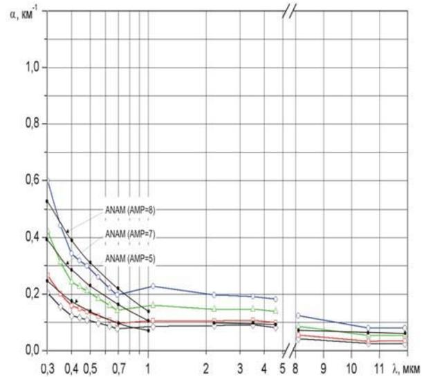
Fig. 5. Aerosol extinction  $\sigma(\lambda)$  spectrum at height  $H = 20$  m for fetch  $X = 3$  km, wind speed  $U = 3.3$  m/s and for various relative humidity:  $\blacklozenge$  -  $RH = 66\%$ ,  $\blacksquare$  -  $RH = 75\%$ ,  $\blacktriangle$  -  $RH = 85\%$ ,  $\bullet$  -  $RH = 90\%$ .
