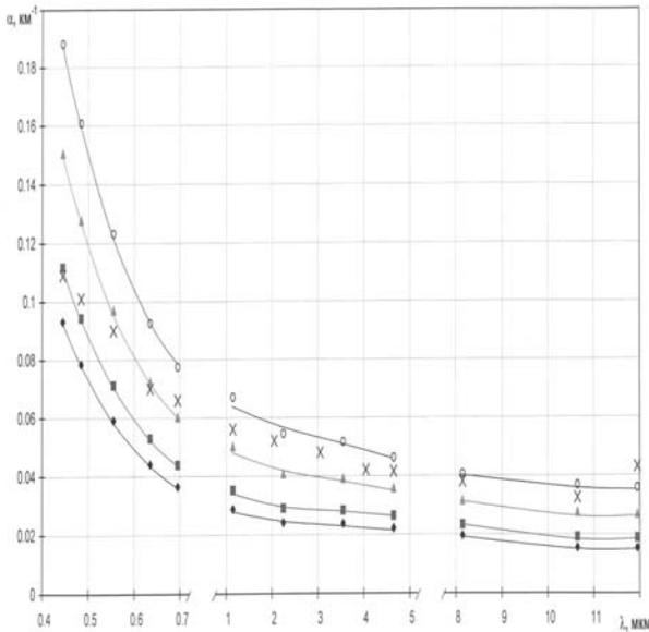
Fig. 4. Aerosol extinction spectrum  $\sigma(\lambda)$  at height  $H = 20$  m for fetch  $X = 30$  km, wind speed  $U = 3.3$  m/s and for various relative humidity:  $\blacklozenge$  -  $RH = 66\%$ ,  $\blacksquare$  -  $RH = 75\%$ ,  $\blacktriangle$  -  $RH = 85\%$ ,  $\bullet$  -  $RH = 90\%$ .
