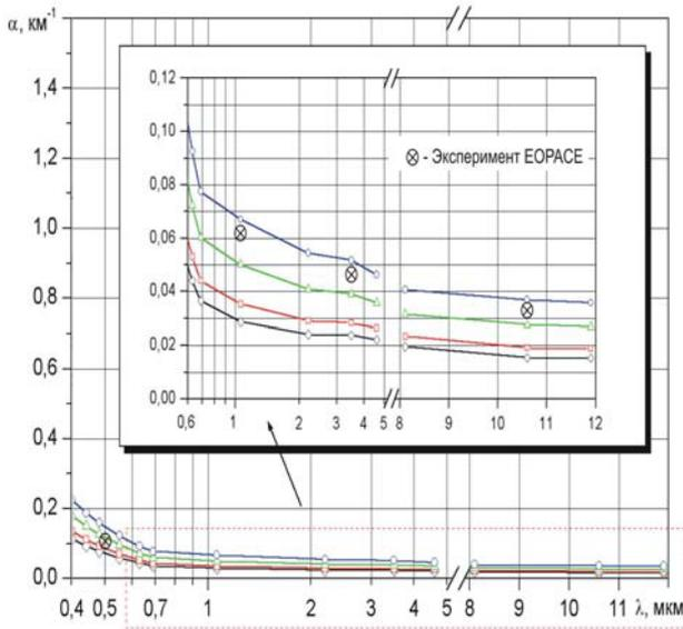
Fig. 6. Aerosol extinction spectrum  $\sigma(\lambda)$  at height  $H = 20$  m for fetch  $X = 30$  km, wind speed  $U = 3.3$  m/s and for various relative humidity:  $\blacklozenge$  -  $RH = 66\%$ ,  $\blacksquare$  -  $RH = 75\%$ ,  $\blacktriangle$  -  $RH = 85\%$ ,  $\bullet$  -  $RH = 90\%$ .
