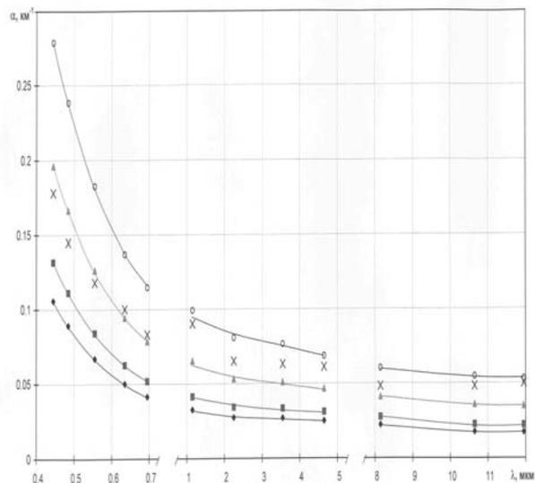
Fig. 2. Aerosol extinction spectrum  $\sigma(\lambda)$  at height  $H = 2.5 \text{ m}$  for fetch  $X = 30 \text{ km}$ , wind speed  $U = 3.3 \text{ m/s}$  and for various relative humidity:  $\blacklozenge$  -  $RH = 66 \%$ ,  $\blacksquare$  -  $RH = 75 \%$ ,  $\blacktriangle$  -  $RH = 85 \%$ ,  $\circ$  -  $RH = 90 \%$ .
