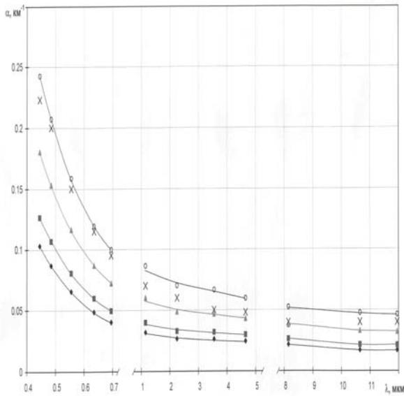
Fig. 3. Aerosol extinction spectrum  $\sigma(\lambda)$  at height  $H = 4$  m for fetch  $X = 30$  km, wind speed  $U = 3.3$  m/s and for various relative humidity:  $\blacklozenge$  -  $RH = 66\%$ ,  $\blacksquare$  -  $RH = 75\%$ ,  $\blacktriangle$  -  $RH = 85\%$ ,  $\bullet$  -  $RH = 90\%$ .
