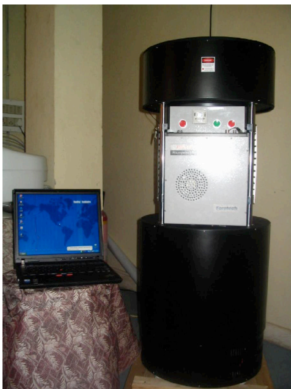
Fig.1. Photograph of Micro Pulse LIDAR at National Physical Laboratory , New Delhi, India
