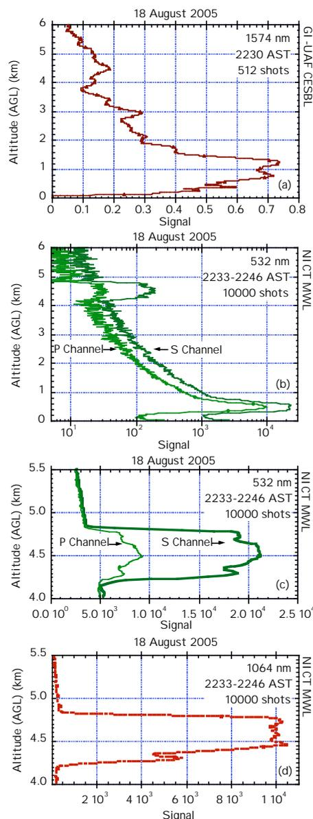
Fig 1. Integrated lidar signals plotted as a function of altitude above ground level. (a) Signal measured by CESBL at 1574 nm. (b) Signal measured by MWL in Channel 4 (s-polarization) and Channel 5 (p-polarization) at 532 nm. (c) Signal measured by MWL in Channel 8 (s-polarization) and Channel 9 (p-polarization) at 532 nm. (d) Signal measured by MWL in Channel 7 at 1064 nm.
