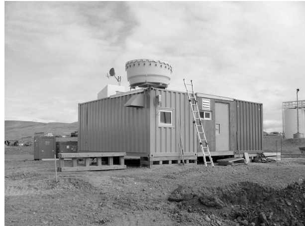
Figure 1. Two seaintainers are joined together as shelter for the lidar, radar, and PAREI instruments. The radar antenna is on the near corner of the shelter and the lidar window is in the white box behind the radar antenna.
