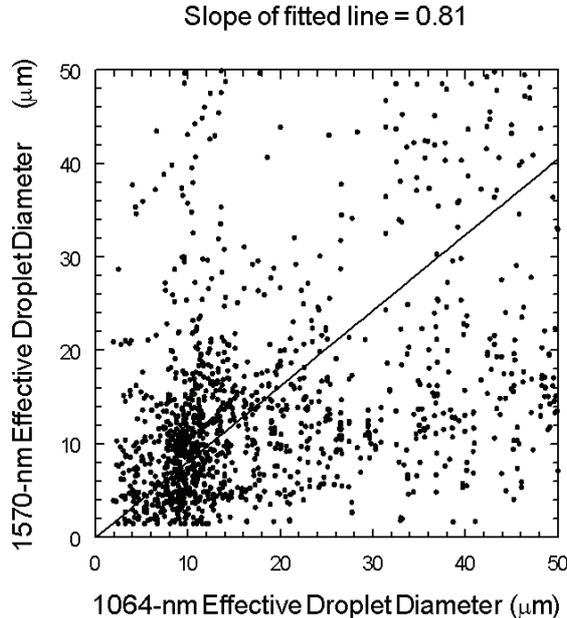
Figure 2. Scatter plot of the effective droplet diameter solution values derived from the MFOV1 and MFOV2 lidars for the vertical soundings recorded on 15 September 2005.
