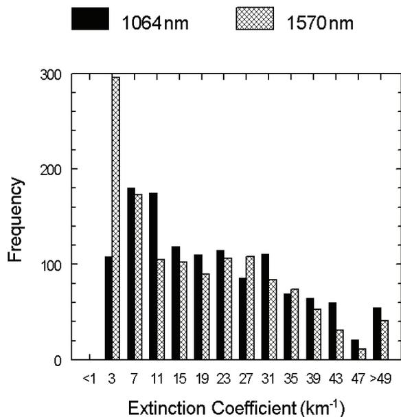
Figure 4. Histograms of the extinction coefficient solution values derived from the MFOV1 (solid) and MFOV2 (patterned) lidars for the vertical soundings recorded on 15 September 2005. Same data as in Fig. 1
