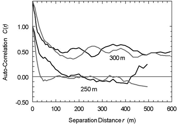
Figure 3. Spatial auto-correlation functions of the fluctuations of the retrieved extinction coefficient (black) and effective droplet diameter (grey) calculated over the 250-m (lower curves) and 300-m (upper curves) horizontal planes cut into the volume scanned by MFOV2 at 12h03 UTC on 15 September 2005. The ordinate for the 300-m curves is shifted upward by 0.5 to improve readability. Cloud base at  $\sim 225$  m.
