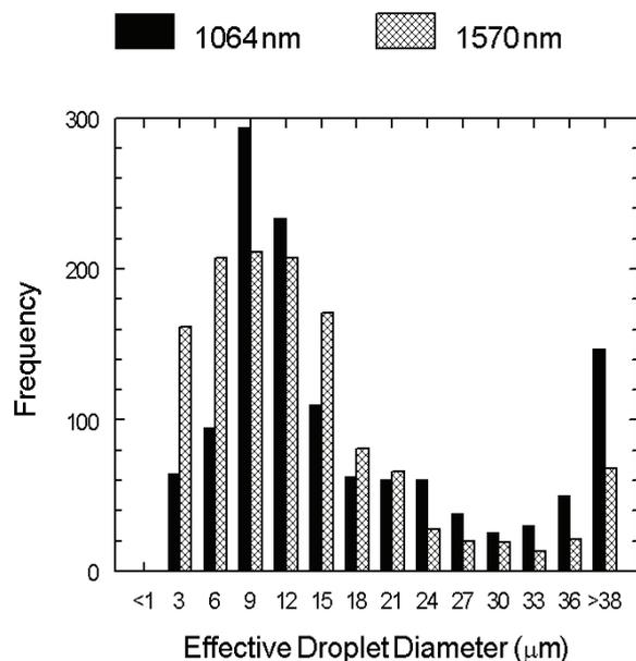
Figure 5. Histograms of the effective droplet diameter solution values derived from the MFOV1 (solid) and MFOV2 (patterned) lidars for the vertical soundings recorded on 15 September 2005. Same data as in Fig. 2.
