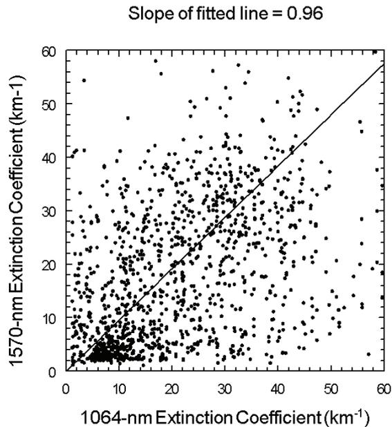
Figure 1. Scatter plot of the extinction coefficient solution values derived from the MFOV1 and MFOV2 lidars for the vertical soundings recorded on 15 September 2005.
