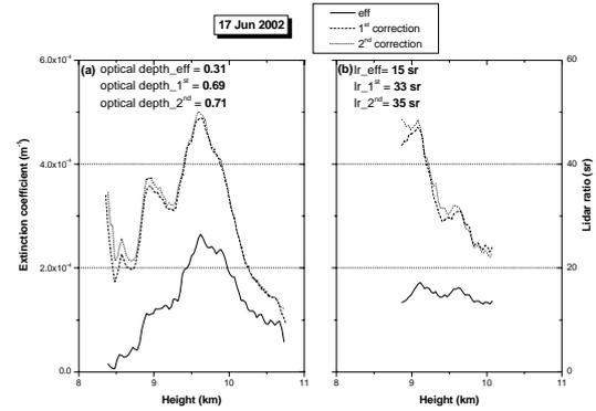
Fig. 3. Profiles of the extinction coefficient (a) and lidar ratio (b) obtained with a Raman lidar. The profiles were corrected for multiple scattering effect
