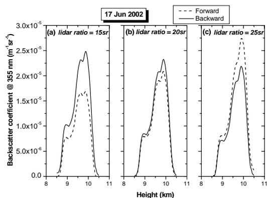
Fig. 1. Forward (dashed curve) and backward backscatter coefficient (solid curve) by assuming lidar ratio of (a) 15sr, (b) 20sr, and (c) 25sr
