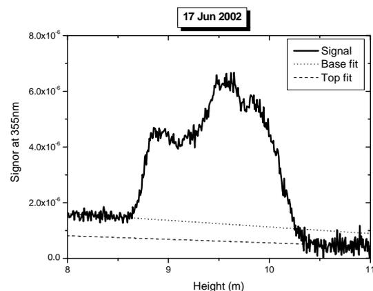
Fig. 2 Lidar-scattering signal fits at the bottom and top of the cirrus cloud
