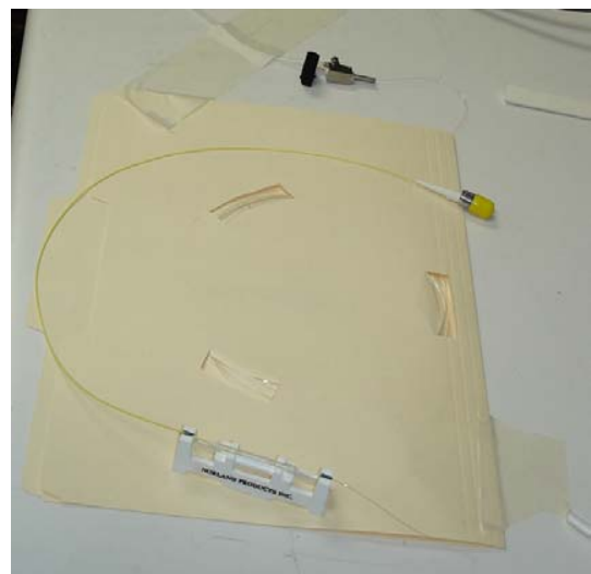
Figure 2 Fiber gas cell used to lock DFB laser. The cell is 5 meters long.
