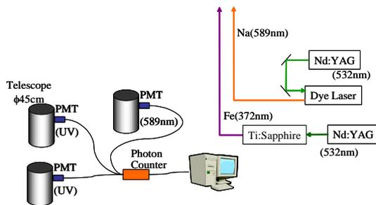
Fig. 1. The block diagram of the lidar system for the observation of the mesosphere metallic atom layer installed in Kototabang.
