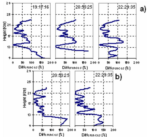
**Fig. 5. Percent of absolute mean differences, between extinction profiles of SAGE II and lidar. a) For 532nm wavelength and b) For 1064nm wavelength.**
