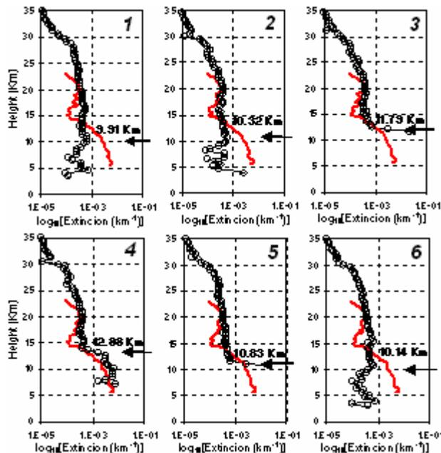
**Fig. 3. SAGE II and CEILAP lidar coincident profiles, corresponding to June 2001 at 532nm.**
