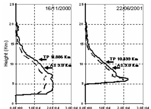
**Fig. 1. Backscatter Aerosols Coefficient, calculated with aerological sounding and density model.**
