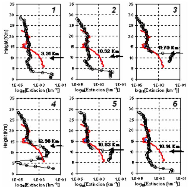
**Fig. 4. SAGE II and CEILAP lidar coincident profiles, corresponding to June 2001 at 1064nm.**
