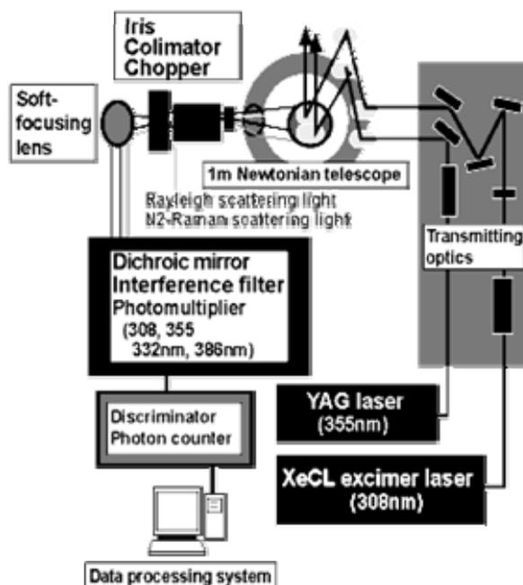
Figure 1. Block diagram of NIES ozone DIAL system
