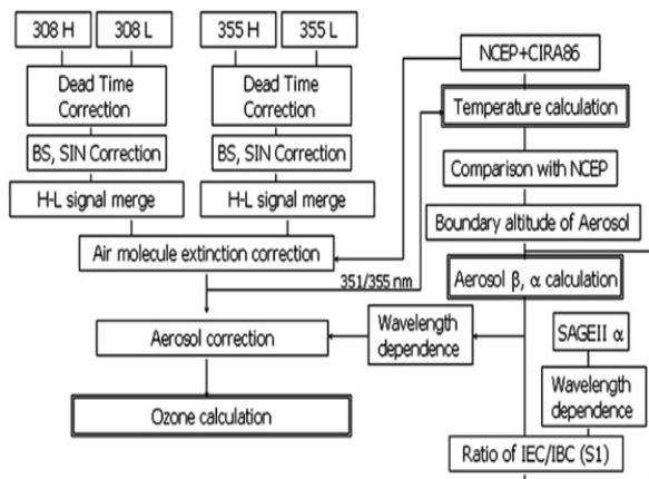
**Figure 2.** Flow chart of signal and data processing
