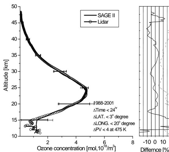
**Figure 4.** Inter-comparison of mean vertical profile between lidar and SAGE II (left) and relative % differences (right)
