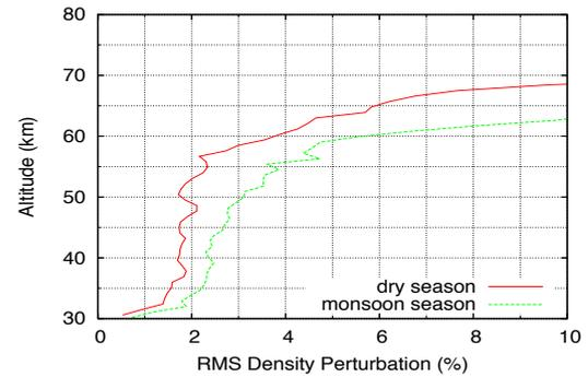
Figure 3. Altitude profile of the average rms atmospheric density perturbations for the dry and monsoon season in 2005, 2006.
