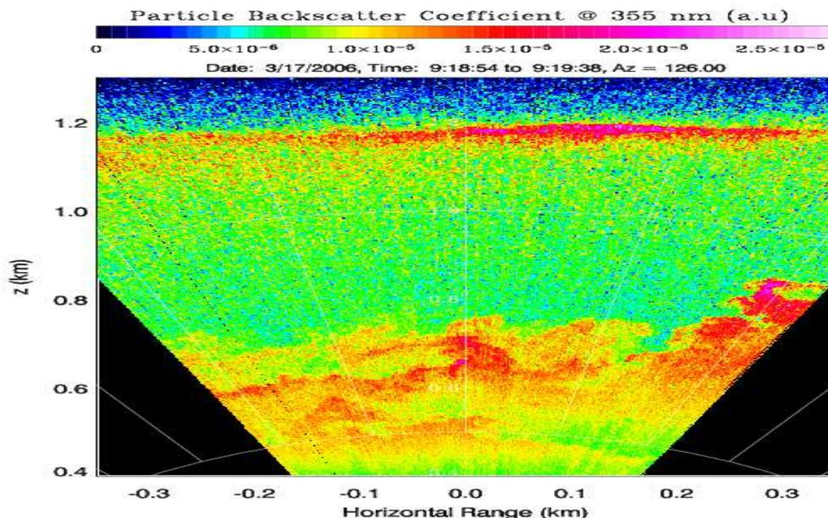
Fig. 4. Aerosol backscatter coefficient of an 45-s RHI sector scan from elevation  $67.5^\circ$  to  $112.5^\circ$ , with a temporal and range resolution of 0.1 s and 3 m, respectively at 355 nm, collected on 17<sup>th</sup> March, 2006, around 09:19 UTC at Stuttgart, Germany. The angular resolution is  $0.1^\circ$ .
