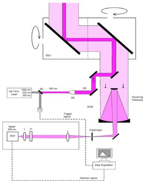
Fig. 1. Set up of the scanning aerosol lidar system of UHOH. BD: beam dump, BE: beam expander, BSU: Scanner (beam steering unit), IF: interference filter, L: lenses, LM: laser mirrors, PMT: photomultiplier tube, BS: Beam Splitter, BSM: Beam Steering Mirror, PD: Photo-Diode.
