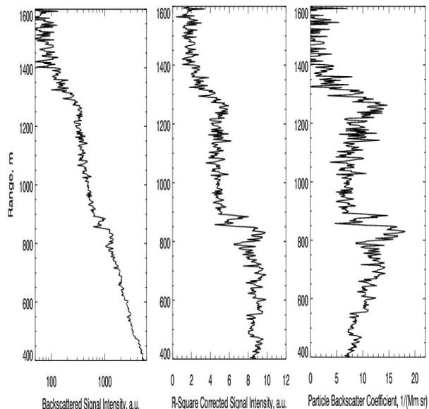
Fig. 3. Retrieval of the aerosol backscatter coefficient at 355 nm. This profile is a 3-shot average of an RHI sector scan collected on 17<sup>th</sup> March, 2006, at 09:19 UTC. The figure represents: the background-subtracted signal (left panel), range-corrected signal (middle panel) and particle backscatter coefficient in  $(\text{Mm sr})^{-1}$  (right panel). A plot of the full RHI scan is shown in Fig. 4.
