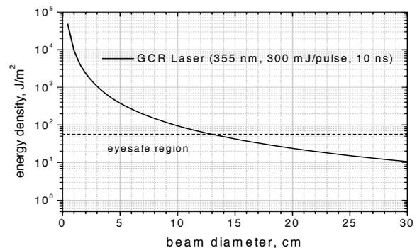
Fig. 2. Eye safety considerations for the scanning aerosol lidar: Energy density against beam diameter, taking the maximum energy density within the inhomogeneous laser beam profile of our Nd:YAG laser into account. The dashed line shows the maximum allowed energy density of 56 J/m<sup>2</sup>. For a diameter larger than 13 cm, our laser beam is eye safe according to DIN (Deutsche Industrie Norm) rules.
