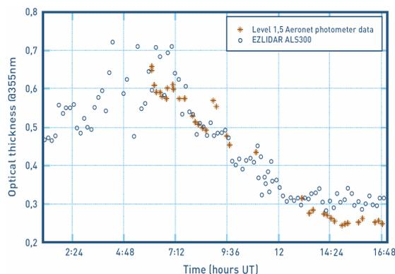
Fig.4. The comparison of the sunphotometer with the Easy Lidar total optical depth. The sunphotometer data (red crosses) were provided by P.Goloub, AERONET, France. The Easy Lidar results (blue dots) were obtained by automated software without need of post processing. Around noon the sunphotometer data were not available due to passing subvisible clouds hindering retrieval.
