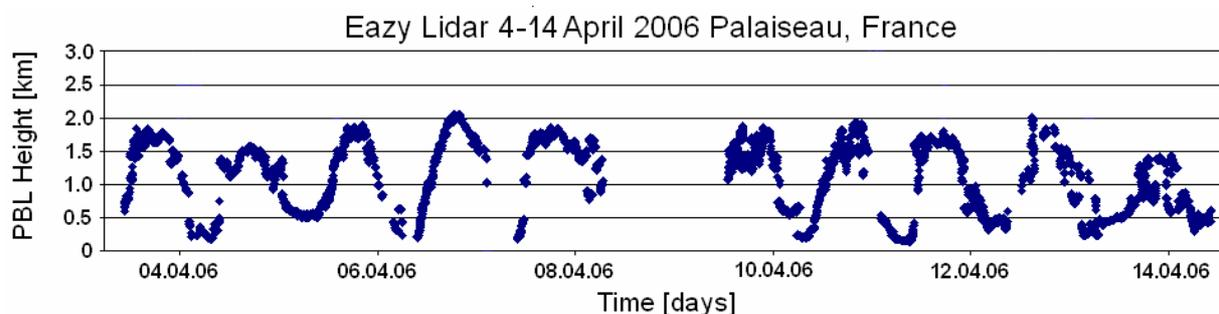
Fig.2. Unattended, continuously running Easy Lidar measurements of the Planetary Boundary Layer height evolution for a period over 10 days in April 2006 at Palaiseau, France. The control software automatically stopped the measurement on midday on 8 May (saturation of the PMT due to low clouds) and restarted on midday on 9 May.
