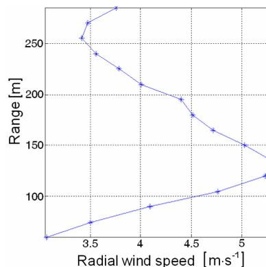
Fig.3. The radial wind speed at 30° with constant range resolution of 15m obtained from the Easy Lidar wind measurement on 15 February 2006 at Palaiseau, France.
