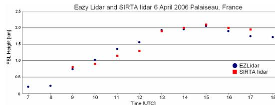
Fig.5. The height of the Planetary Boundary Layer obtained on 6 April 2006 from the near field 532nm SIRTA lidar measurements (red squares) provided by M.Haefelin, SIRTA, Palaiseau, France agree well with the 355nm Easy Lidar results (blue dots).
