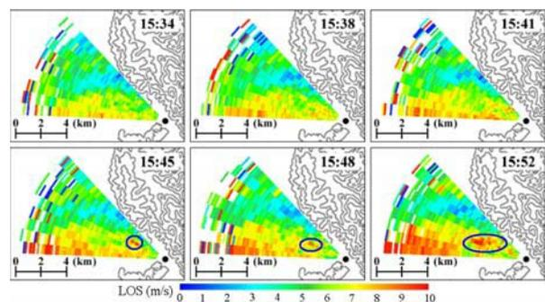
Fig. 3. PPI scan of the LOS wind speed along the Mogami valley at 15:34-15:52 JST on August 30, 2004. The two-axis scanning device was set to scan between 275 and 315° in azimuth at an elevation angle of 25°. The elevation angle was stepped in 5° increments. The laser pulse accumulation was 1000 for the each azimuth angle. It took three and half minutes to obtain one PPI scan.
