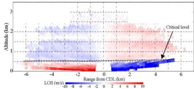
Fig. 2 RHI scan of the LOS wind speed along the Mogami valley at 9:22-9:42 JST on August 30, 2004. The two-axis scanning device was set to scan between 0 and 90° in elevation at azimuth angles of 135° and 315°. The elevation angle was stepped in 2° increments. The laser pulse accumulation was 500 for the each elevation angle. It took about twenty minutes to obtain one RHI scan. Blue shows towards the CDL, and red shows away from the CDL.
