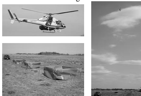
Fig.3 Views of the helicopter-based fluorescence lidar observation with the target of three portable pools.
