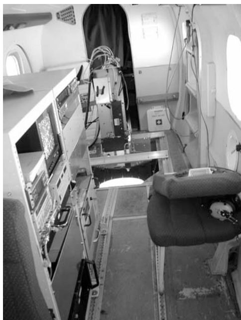
Fig. 1. Photograph of NOAA Fish LIDAR in NOAA Twin Otter. The rack on the left contains laser power supply and cooling system, computer, and timing electronics. The optics package with laser and receiver is aft of the rack, just to the right in the photo.
