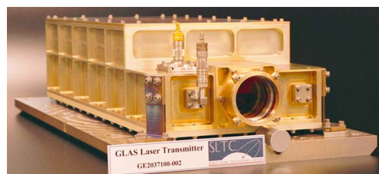
Fig. 3. External photograph of the GLAS laser serial number 2. Visible is the output port of the laser beam, the mounting flexures, quick disconnects (remove before flight) for venting and purging with air, and a reference mirror used to align the pointing of the laser beam referenced to the mounting feet.
