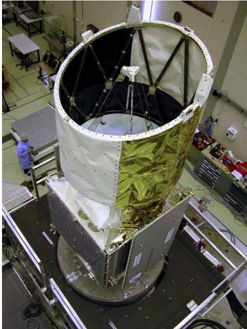
Fig.3. Structural Model Satellite being prepared for vibration testing
