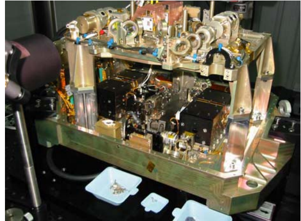
Fig. 2. Engineering Qualification Model of Power Laser Head (Upper optical bench mounted on temporary stand-offs)
