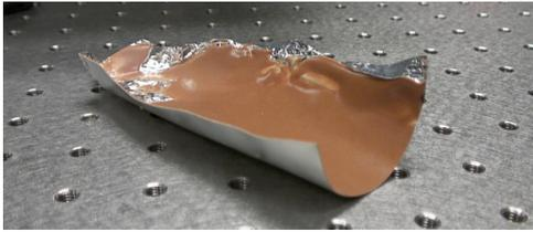
**Figure 3 Sample used for contamination testing. The above image shows A12 deposited on a 3mm-thick aluminium sheet.**
