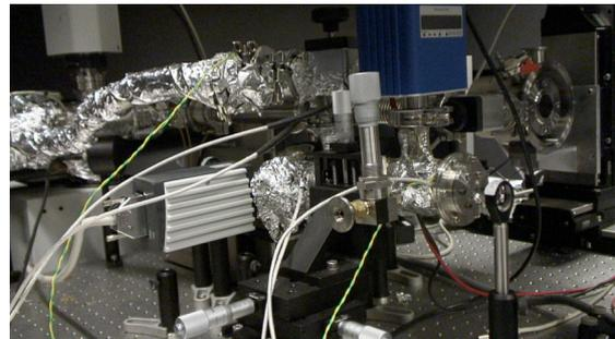
**Figure 2 Vacuum chamber used for contamination experiments. The picture is taken during bake-out, with the fused silica windows replaced by aluminium blanks.**
