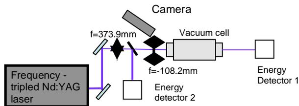
**Figure 1 Experimental setup to investigate the contamination effect of space materials containing hydrocarbons and silicones.**
