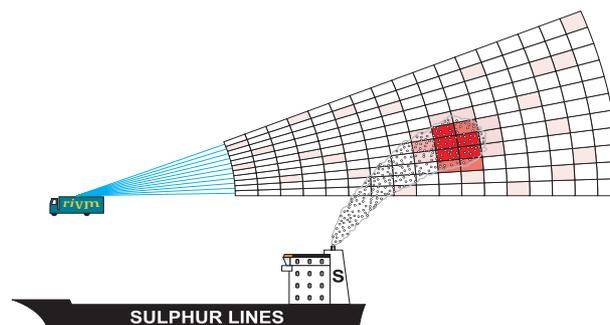
Fig. 9. Overview of measurement of ship emission.
