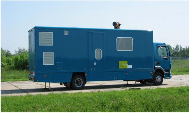
Fig. 4. The mobile lidar system, while measuring.
