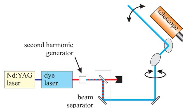
Fig. 1. Simplified scheme of the lidar system.
