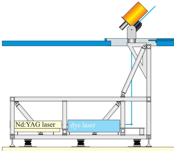
Fig. 5. Frame with emitter and receiver units, with the telescope platform in the elevated position.
