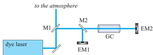
Fig. 3. The spectrophotometer unit, M1: beam sampler, reflectance 1%, M2: beam splitter, reflectance circa 50%, EM1, EM2: energy meters, GC: gas cell, filled with the trace gas under investigation.
