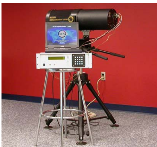
Fig. 2. Photograph of the depolarization lidar. It is equipped with a motorized azimuthal scanner and the whole assembly is mounted on a tripod.
